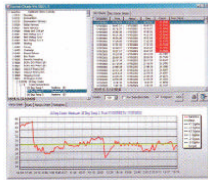
One reporting feature of the Hazard Analysis Tool Series: Graph shows Statistical Process Control of cooler temperatures.
